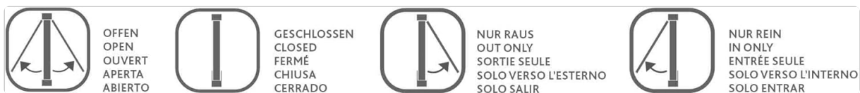
Image 3: Visual representation of the four locking positions: Open, Closed, Out Only, and In Only.
