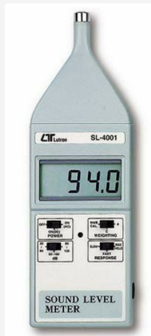
Figure 1: Front view of the SL-4001 Digital Sound Level Meter, showing the LCD display and control switches.
