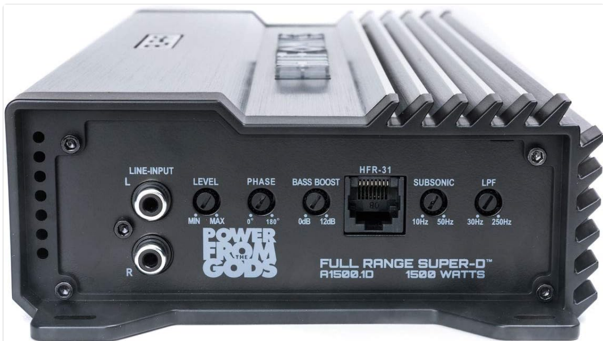
Figure 3: View of the input and control panel of the Hifonics A1500.1D amplifier, showing the RCA line inputs, Level, Phase, Bass Boost, Subsonic, and LPF controls, along with the remote bass control port.
