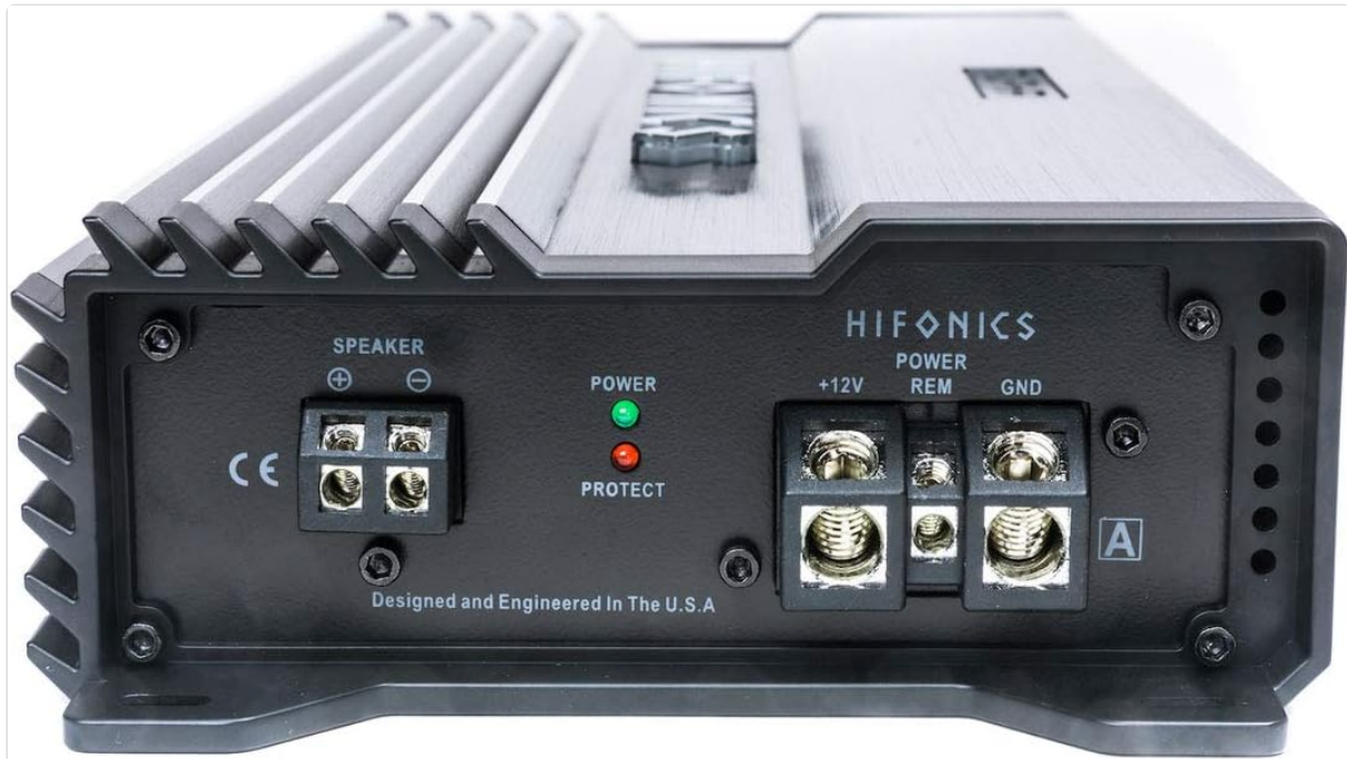
Figure 2: Close-up view of the power input (+12V, REM, GND) and speaker output terminals on the Hifonics A1500.1D amplifier. The green 'PWR' and red 'PRT' indicator lights are also visible.
