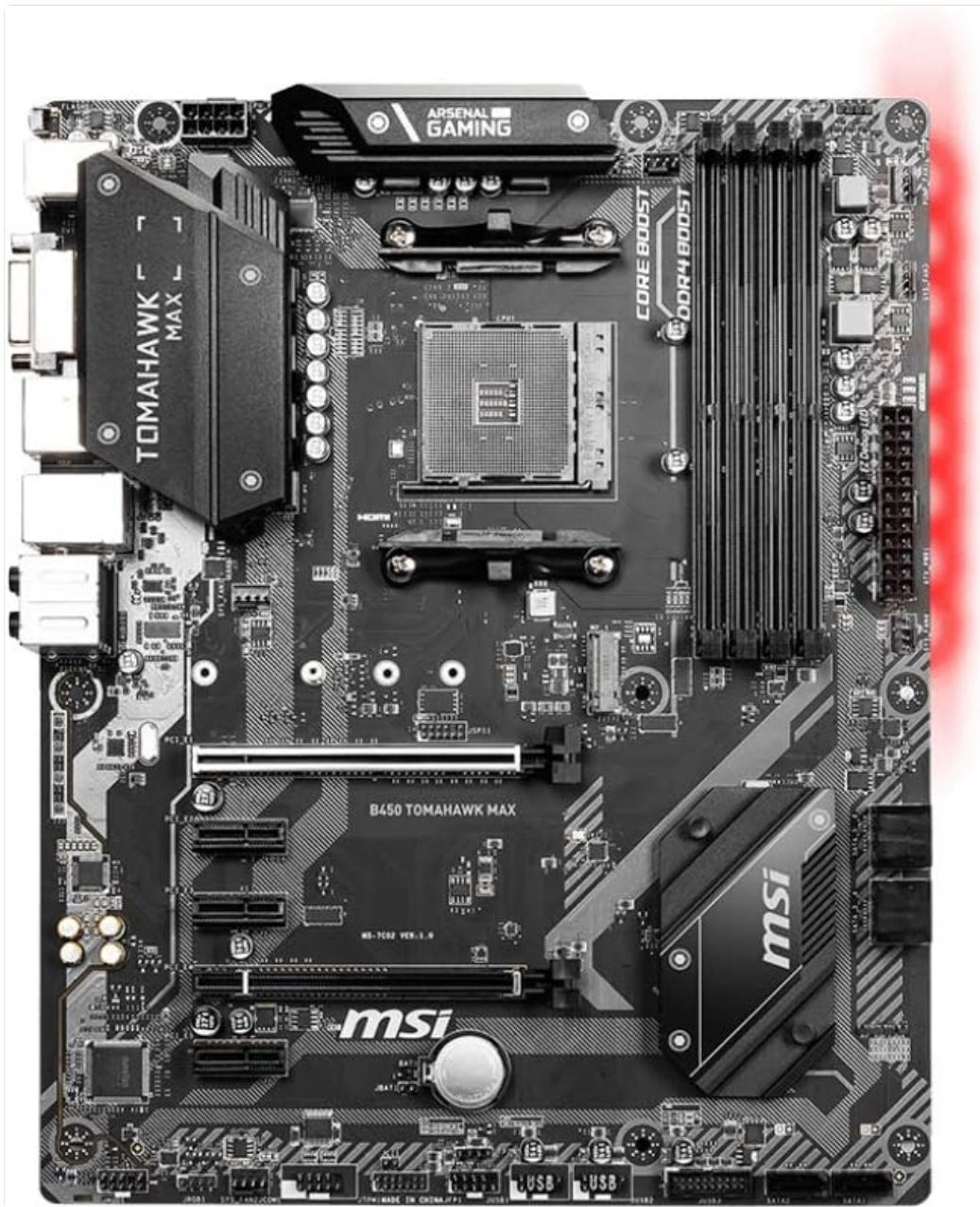
Figure 2.1: Top-down view of the MSI B450 TOMAHAWK MAX motherboard, highlighting key components like the CPU socket, RAM slots, and PCIe slots.
