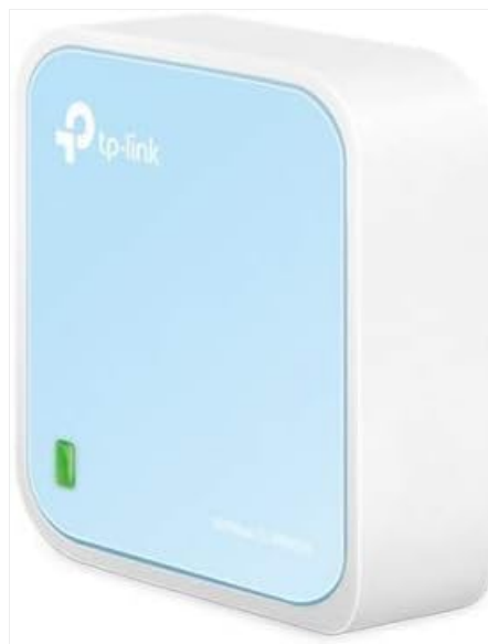
Figure 1: Front view of the TP-Link TL-WR802N Nano Router, showing its compact size and indicator light.
