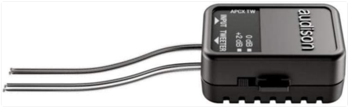
Figure 5: Side view of the Audison APCX TW 570 Crossover, showing its input and output terminals.
