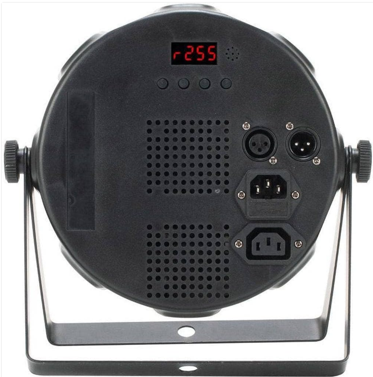
Image: Rear panel of the LP 42 RGBW, highlighting the LED display, control buttons, 3-pin DMX In/Out, and IEC power In/Out connections.
