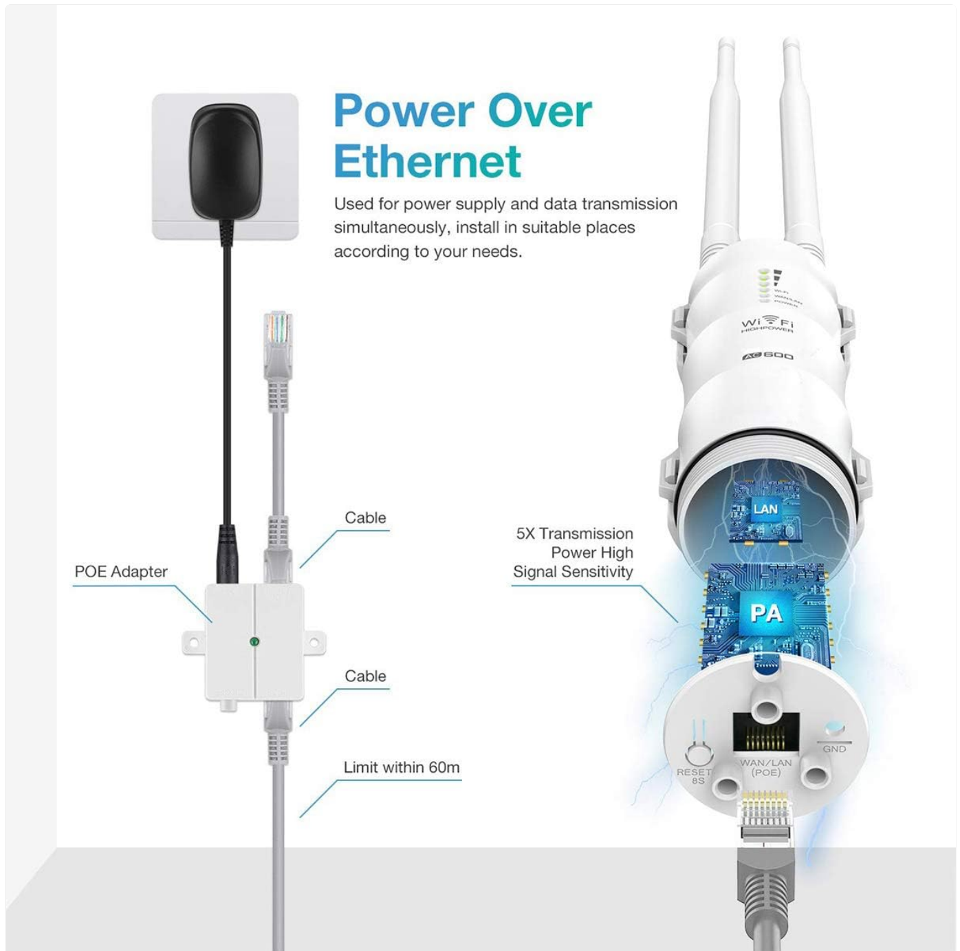
Figure 3.2.1: Diagram illustrating the Power over Ethernet connection setup.
