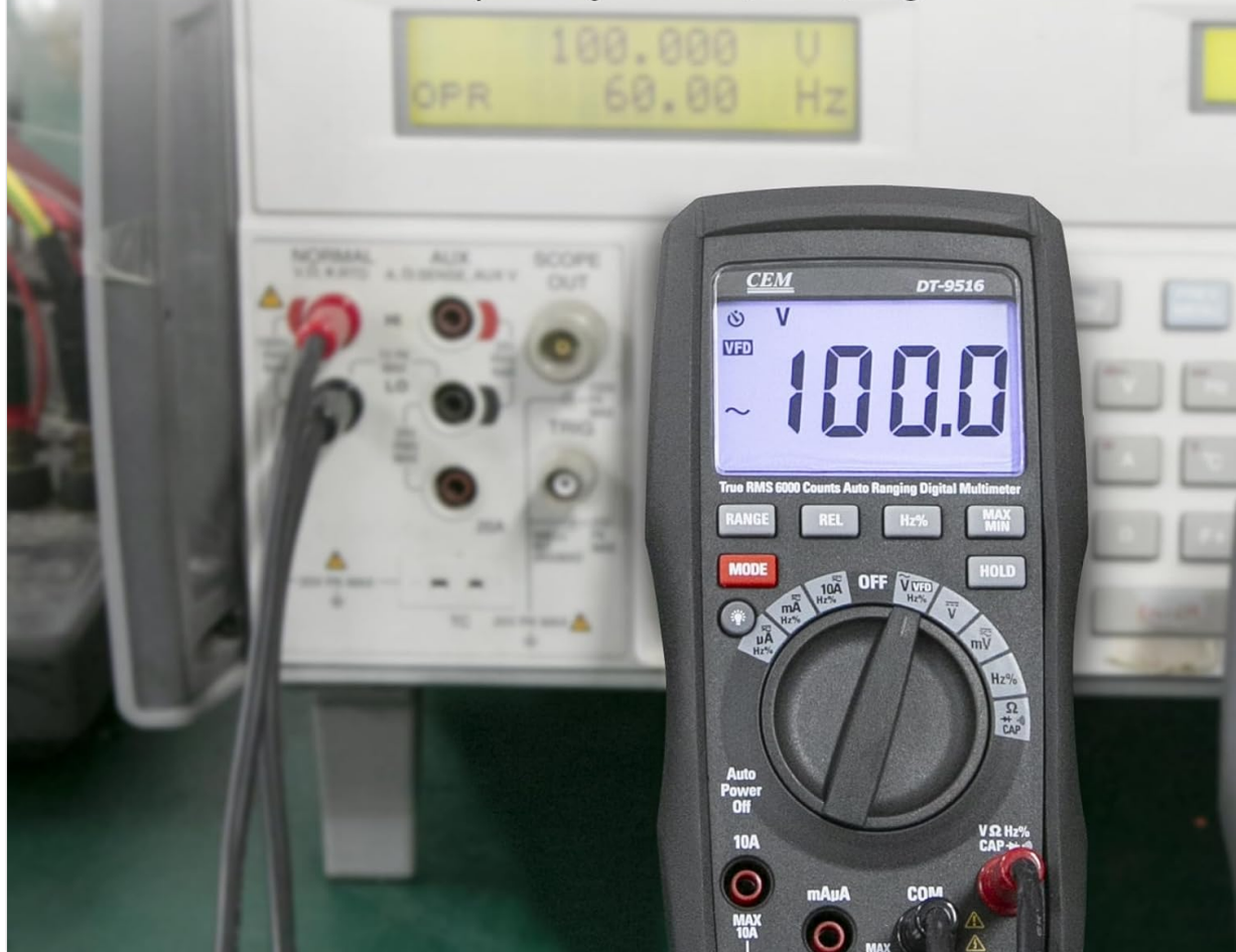
Figure 6: The 6000-count display provides higher resolution and more accurate readings.
