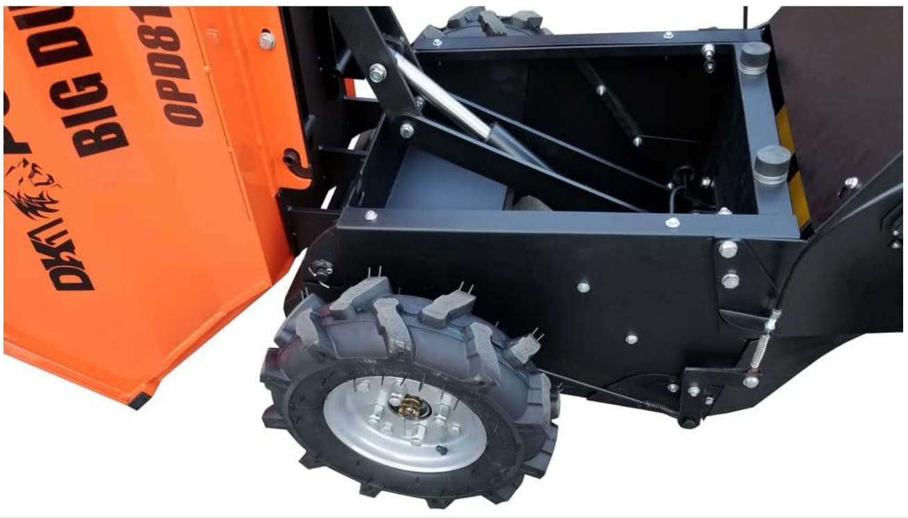
Figure 3.4: Detail of the front pneumatic caster wheels, which allow for easy steering.
