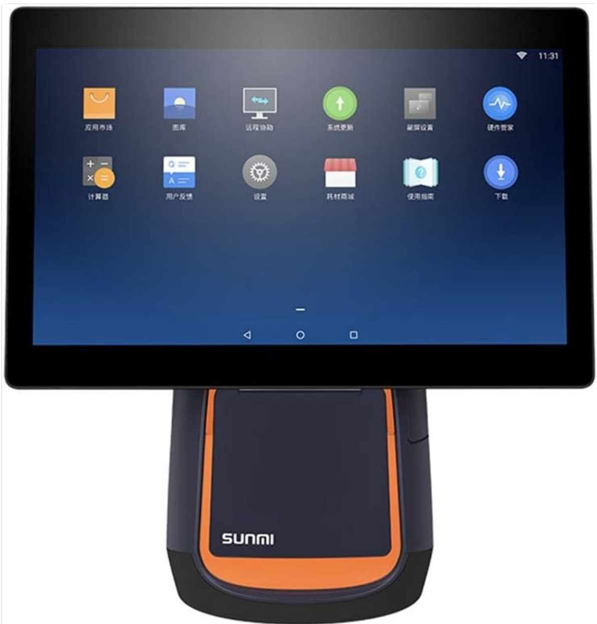
Figure 2.1: Front view of the SUNMI T2 Smart POS Terminal. The 15.6-inch touch screen is visible, displaying various application icons, indicating its Android operating system interface.
