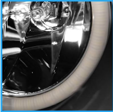
Image 4.2: Detailed views of LED halo, DOT marking, and projector lens.
