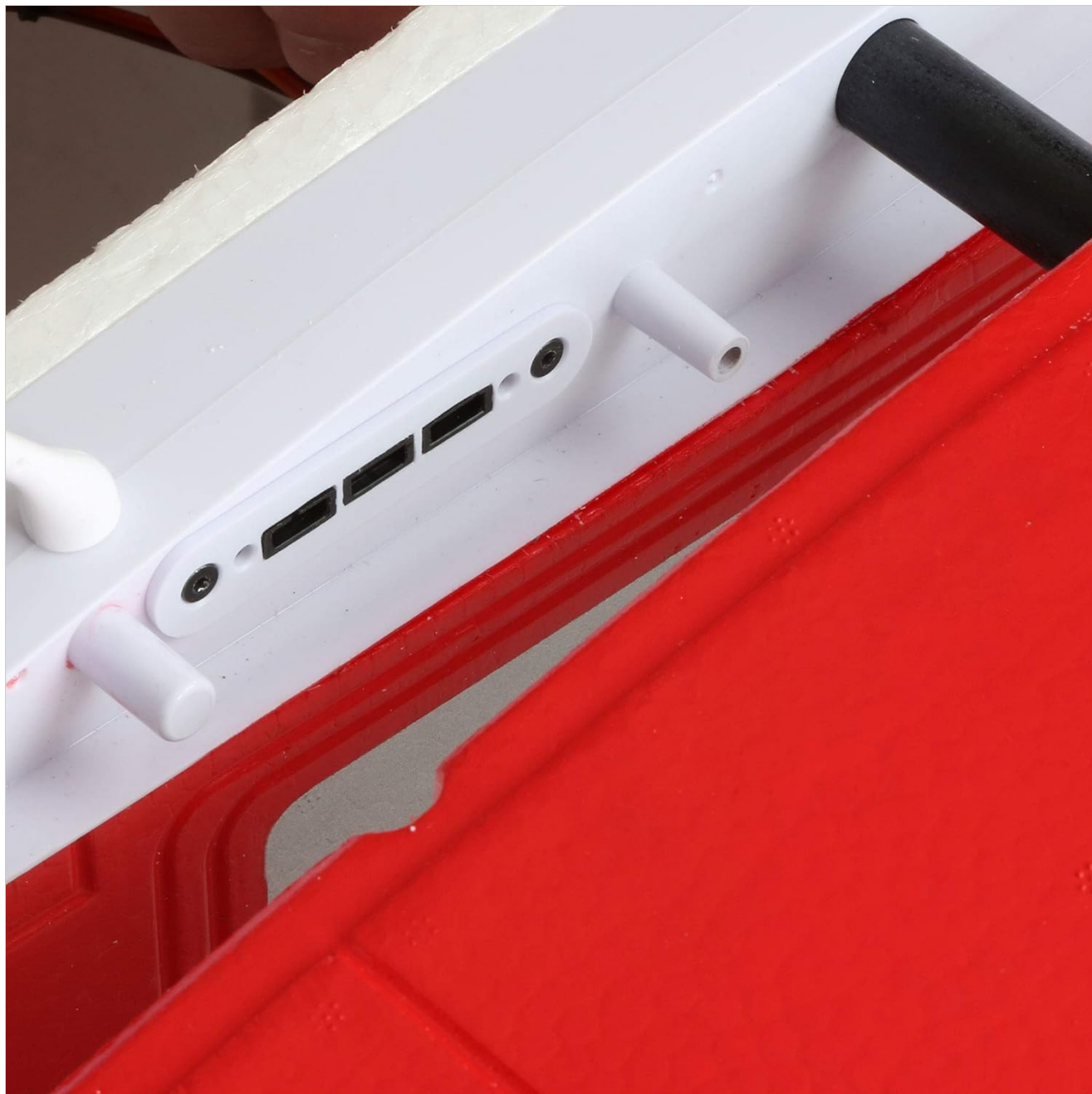
Figure 4.2: Detail of the hands-free servo connection system.
