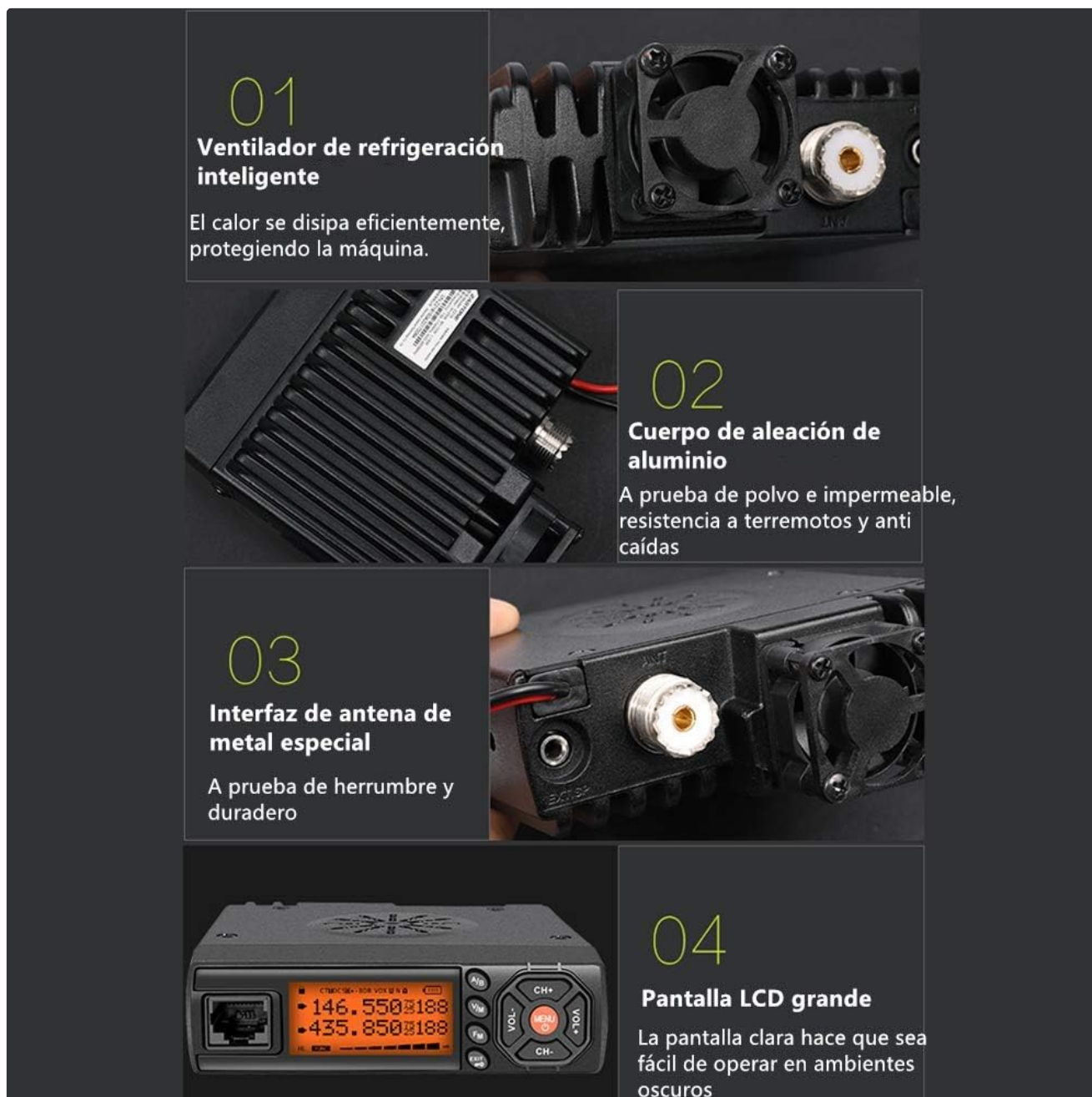
Figure 3.1: Key features of the Zastone Mini Z218, including cooling, construction, and display.
