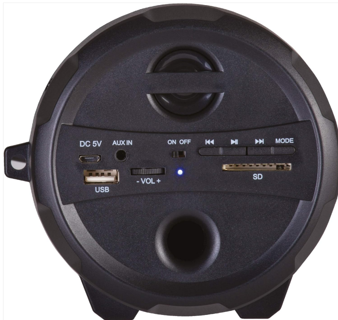
A close-up view of the speaker's control panel, featuring the DC 5V charging port, AUX IN port, ON/OFF switch, USB port, volume controls, track navigation buttons (Previous, Play/Pause, Next), Mode button, and Micro SD card slot.
