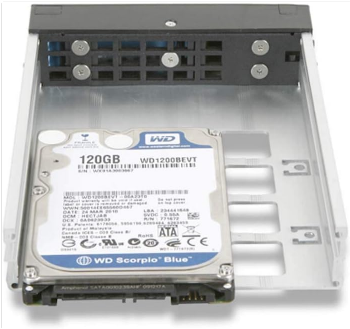
Figure 5: A 2.5" hard drive being inserted into the hot-swap rack.
