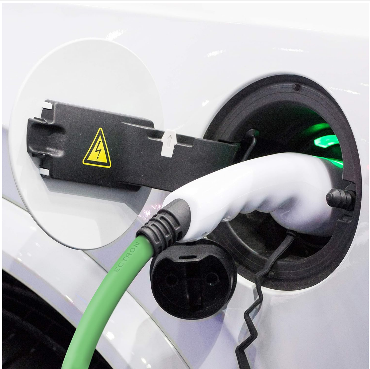
Image 4: Charging Cable Connected to an Electric Vehicle. This image illustrates the Type 2 connector securely plugged into the charging port of a white electric vehicle.
