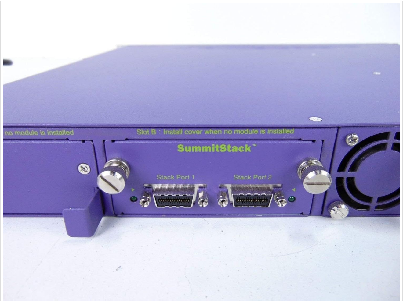
This image displays the rear panel of the Summit X460-24p switch, highlighting the power input, fan modules, and the SummitStack ports. The overall chassis is purple.
