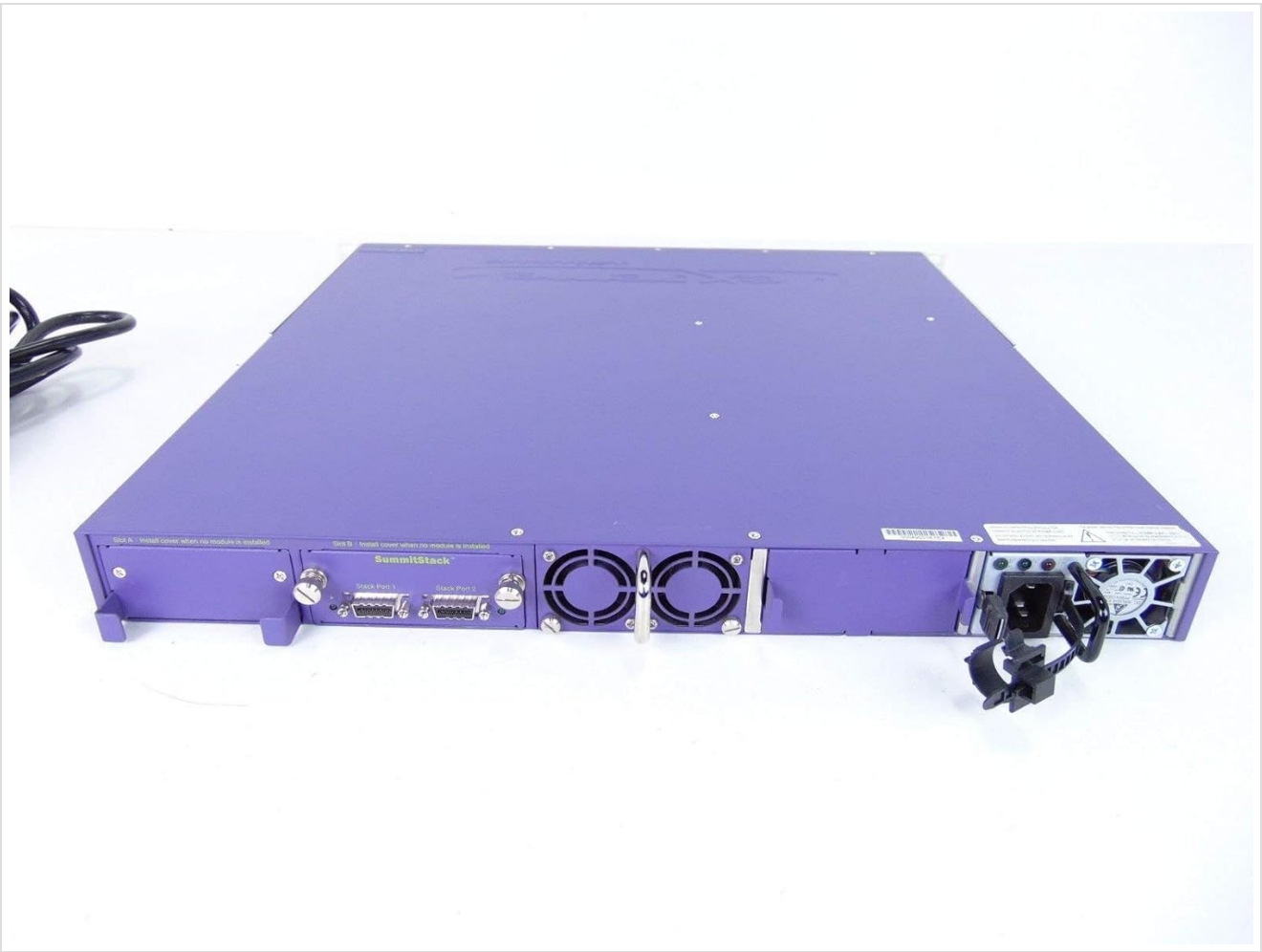
This image displays the rear panel of the Summit X460-24p switch, highlighting the power input, fan modules, and the SummitStack ports. The overall chassis is purple.
