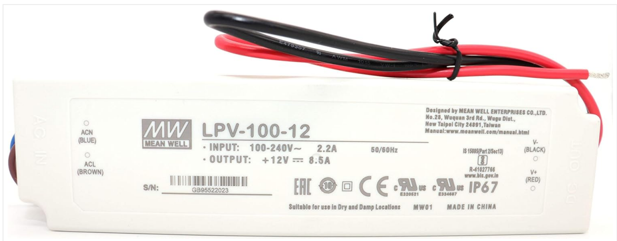
Figure 3.2: Close-up of the product label on the LPV-100-12. The label details input voltage (100-240V~, 2.2A, 50/60Hz), output voltage (+12V == 8.5A), and various certifications including CE, cURus, and IP67.
