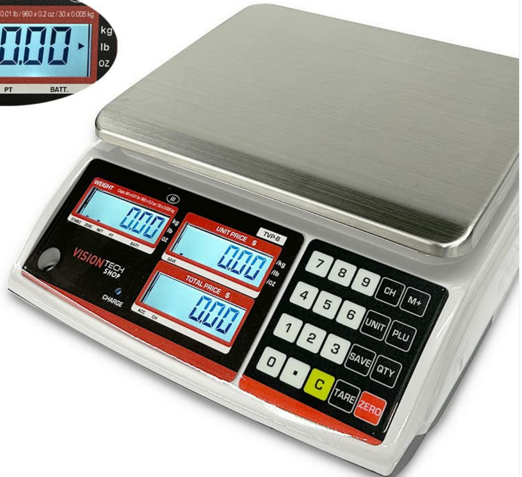
Figure 3: LCD display showing weight and unit options (Lb/Oz/Kg).
