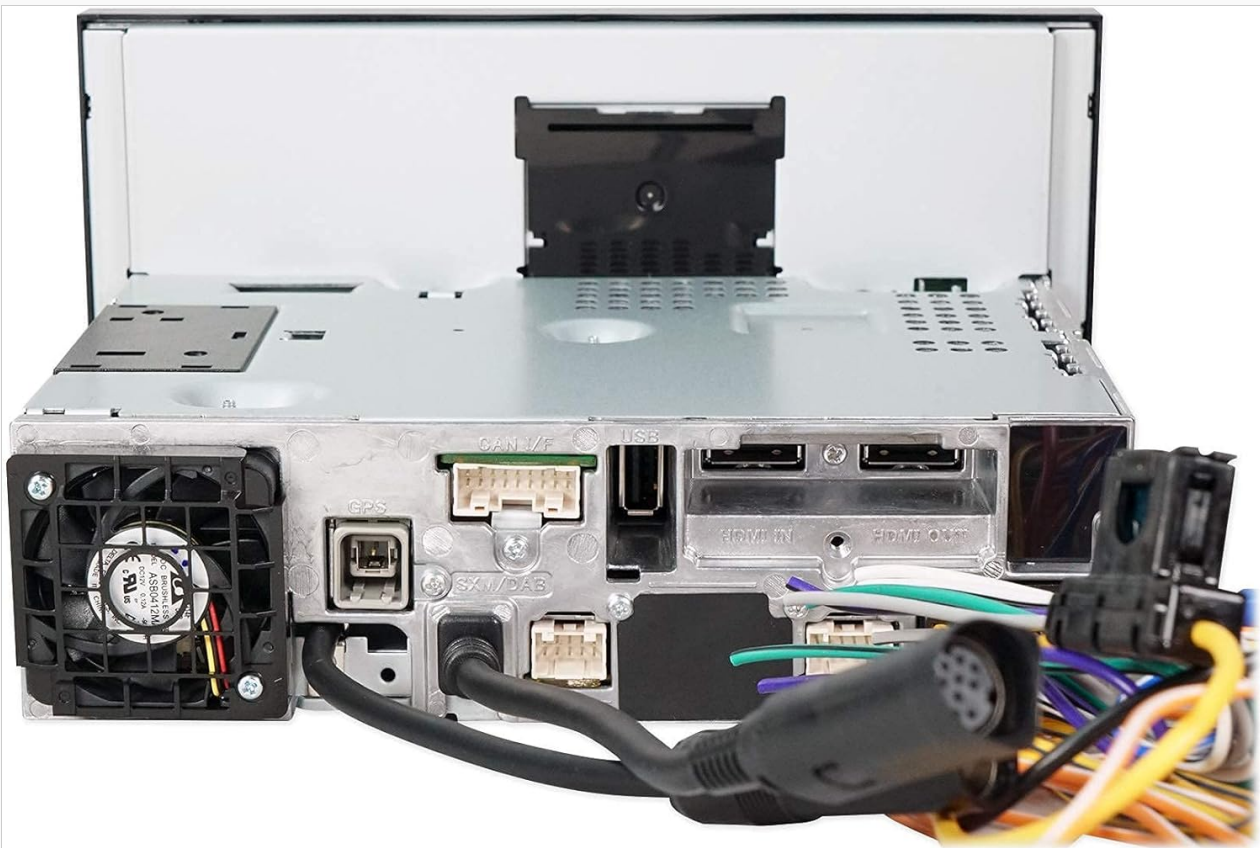
Figure 2.4: Rear Panel Connections. This image provides a detailed view of the rear panel of the Alpine X308U, highlighting its various input and output ports. Visible connections include GPS antenna input, USB ports, HDMI In, HDMI Out, and the main wiring harness connector. A cooling fan is also visible on the left side, indicating thermal management features.
