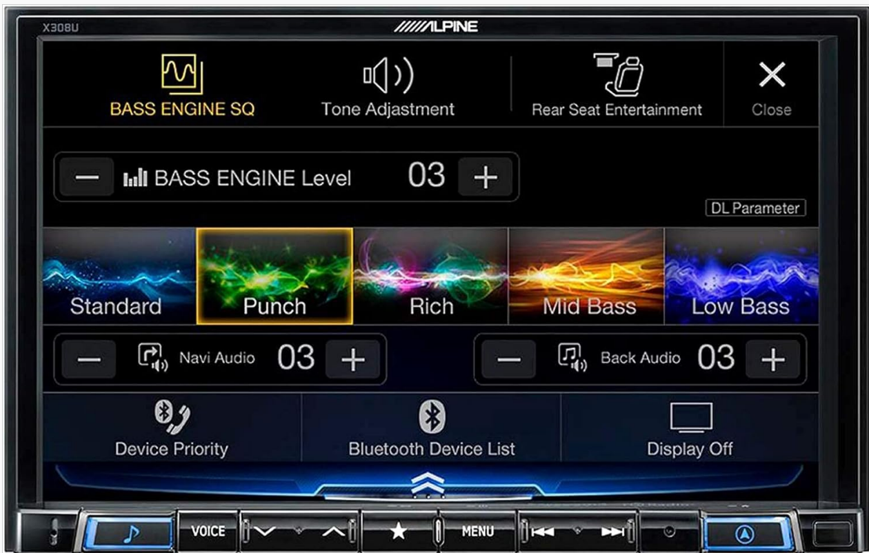
Figure 2.3: Audio Settings Interface. This image displays the "BASS ENGINE SQ" audio adjustment screen on the Alpine X308U. Users can select from various sound presets like Standard, Punch, Rich, Mid Bass, and Low Bass, and adjust levels for Bass Engine, Navi Audio, and Back Audio. This interface demonstrates the unit's comprehensive audio customization options.
