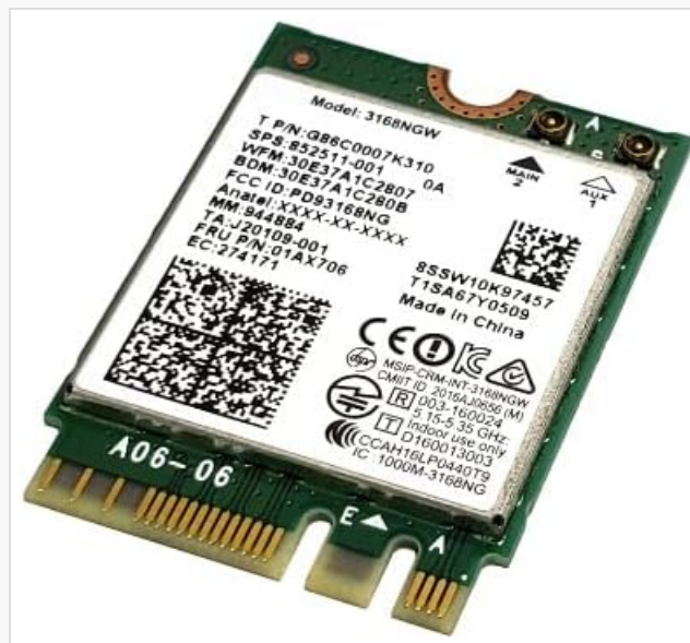
Image 1: Intel 3168NGW Dual Band Wireless-AC 3168 WiFi Card. This image displays the Intel 3168NGW WiFi card, an M.2 2230 form factor component. The card features a green PCB with a white label detailing the model number (3168NGW), part numbers (G86C0007K310, 852511-001), and regulatory information. Two small gold antenna connectors are visible at one end, labeled "MAIN" and "AUX". The M.2 connector pins are visible at the opposite end.
