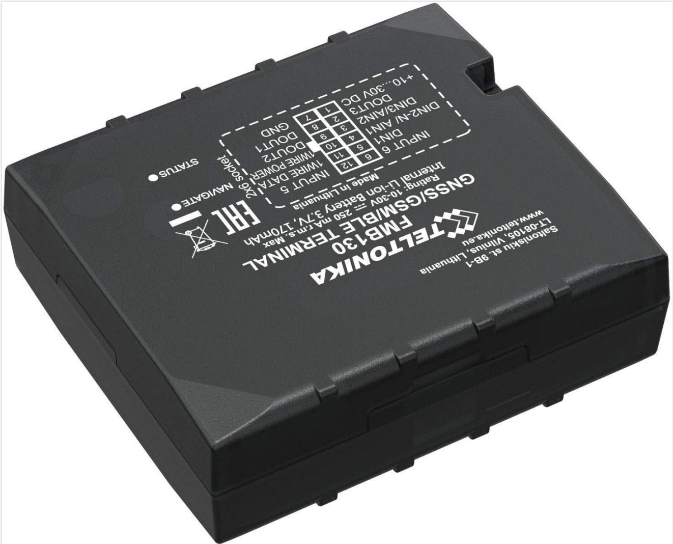
Image: Angled view of the Teltonika FMB130, clearly displaying the pinout labels on the device's casing. This image is helpful for identifying the correct connections for installation.
