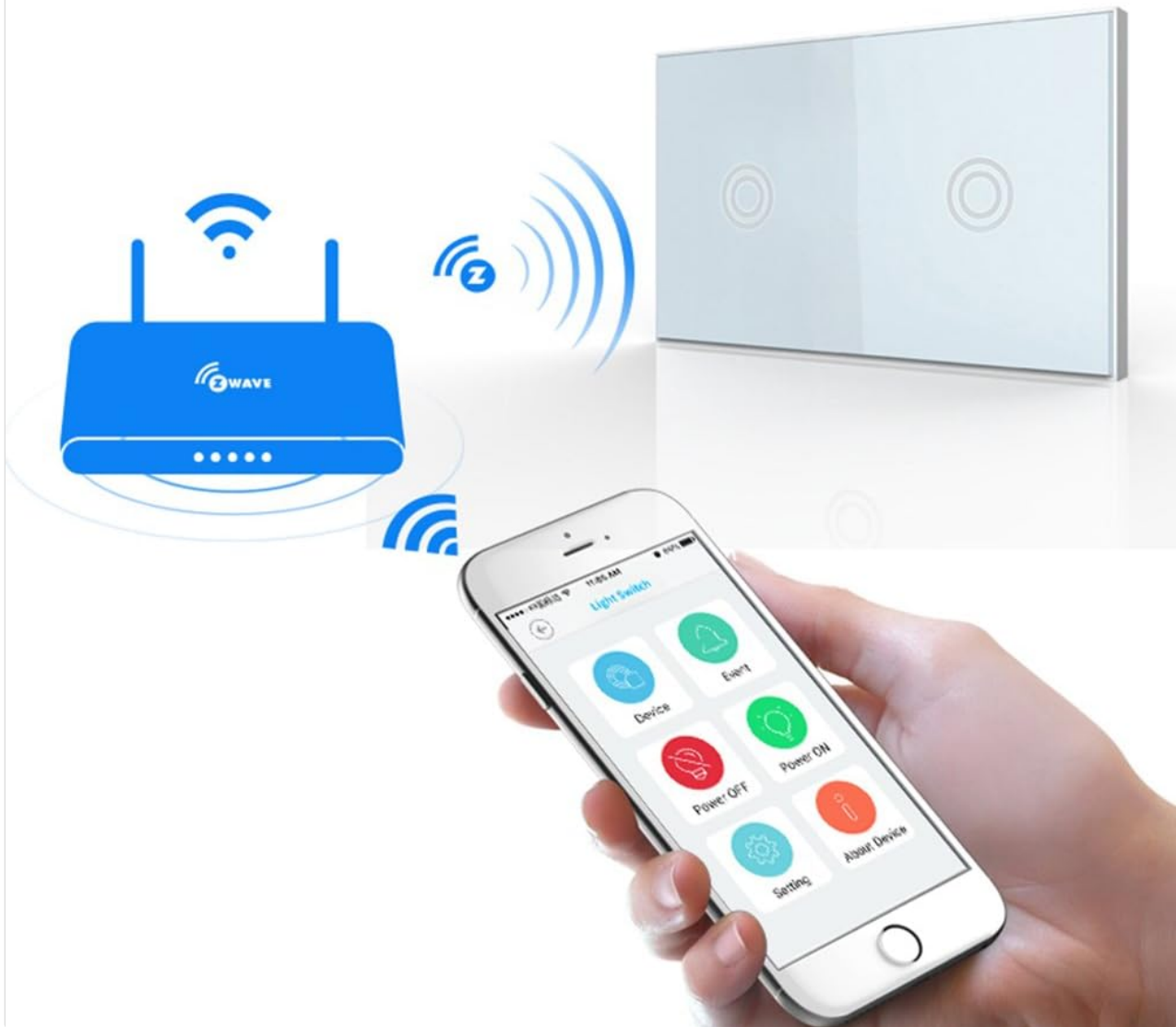
Figure 6.2: Illustration of a smartphone app controlling the smart light switch through a Z-Wave hub, enabling remote management.
