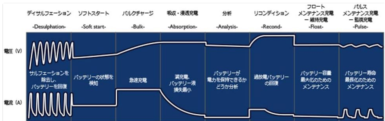
Figure 4: Diagram showing the 8-step charging process, including desulphation, soft start, bulk, absorption, analysis, recond, float, and pulse maintenance stages.
