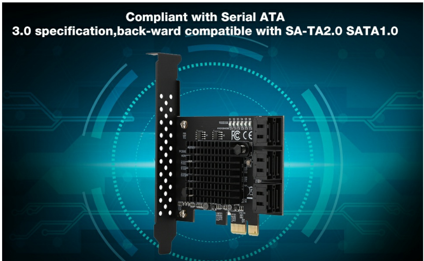
Image 5: Top-down view of the PCE6SAT-M01 card, showing the PCI-Express connector and SATA ports.
