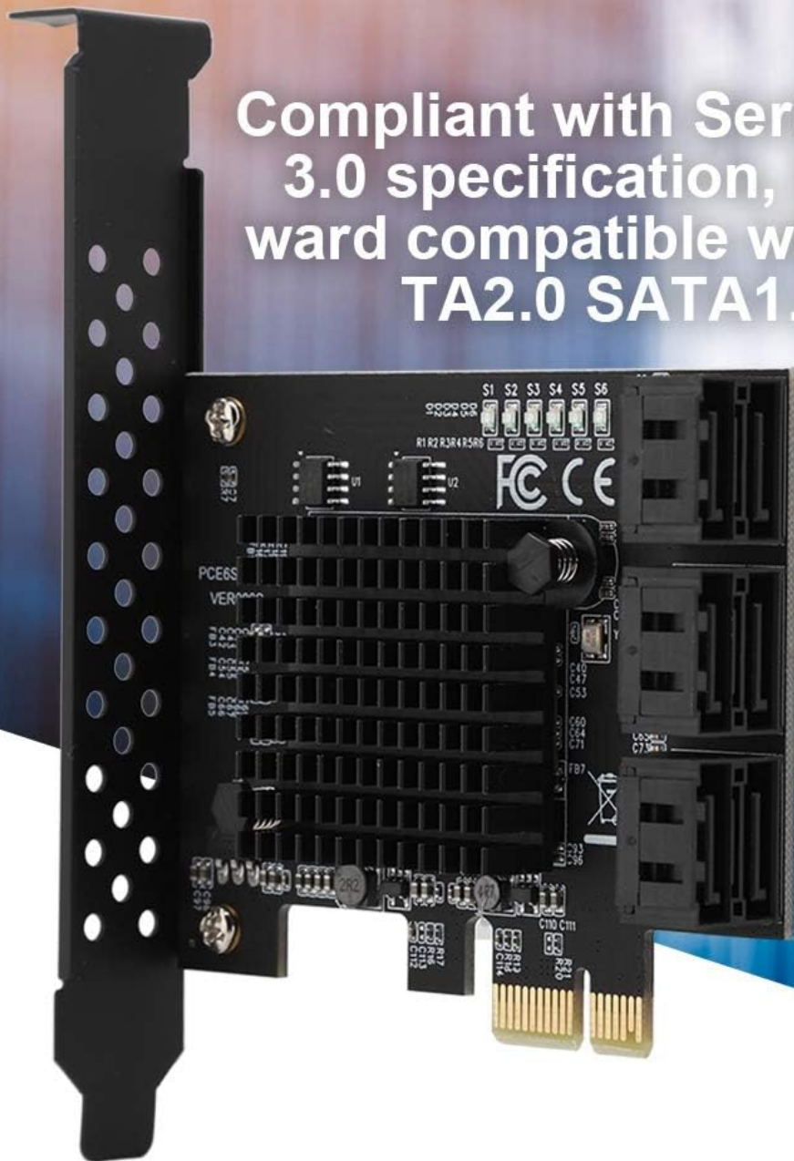
Image 3: The card is compliant with Serial ATA 3.0 specification and backward compatible with SATA 2.0 and SATA 1.0.
