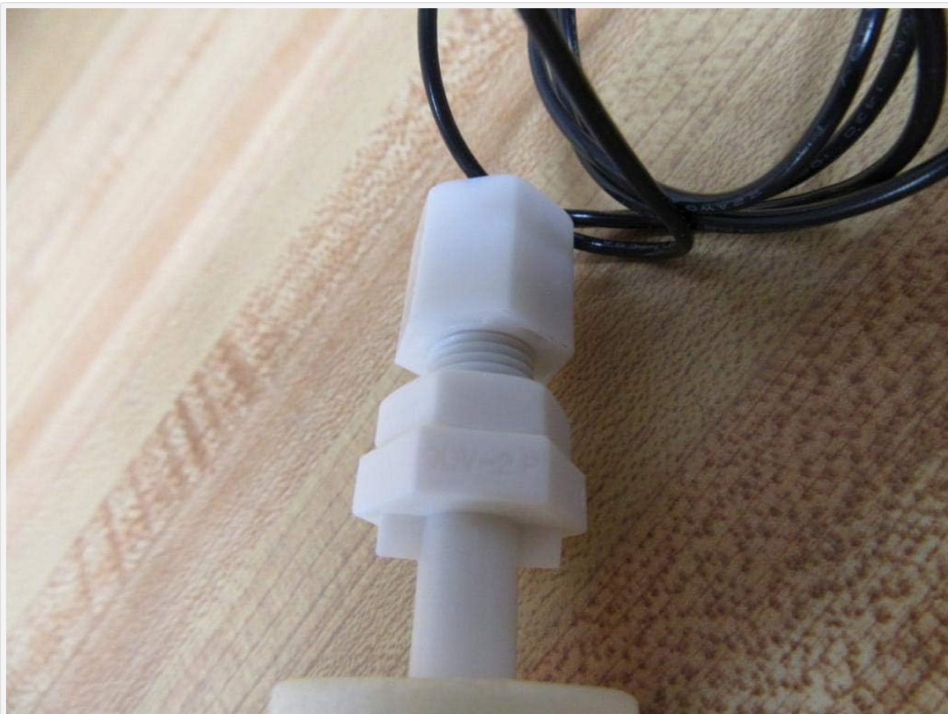
Figure 2: A detailed view of the sensor's threaded connection, indicating how it can be secured.
