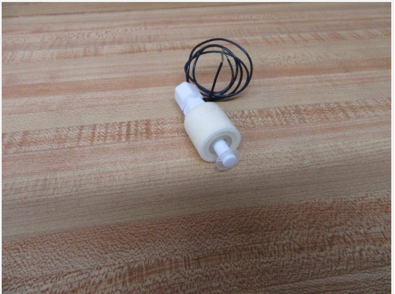
Figure 4: An overhead perspective of the sensor, highlighting the float and the electrical wiring.
