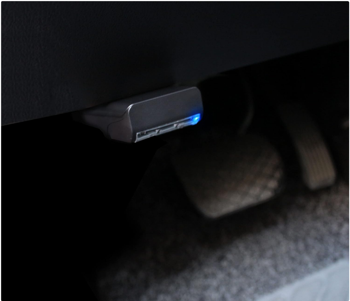
Image 4.1: The RA003 device installed in a vehicle's OBD-II port, typically located under the dashboard.
