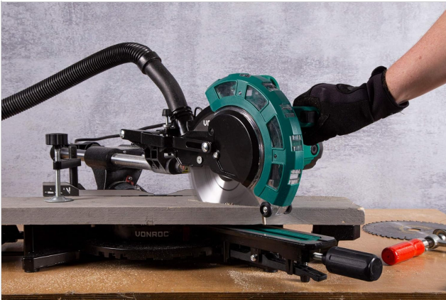
Image 6.1: Demonstrating a cut with the saw, showing proper hand placement and dust extraction hose.
