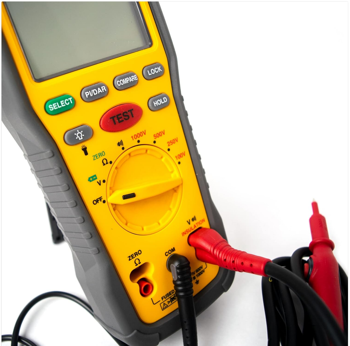
Image 6.2: A close-up view of the test leads securely connected to the IRT803's input terminals.
