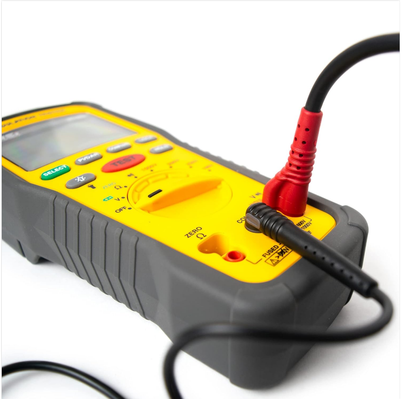
Image 5.1: The IRT803 with test leads properly connected to the input jacks.
