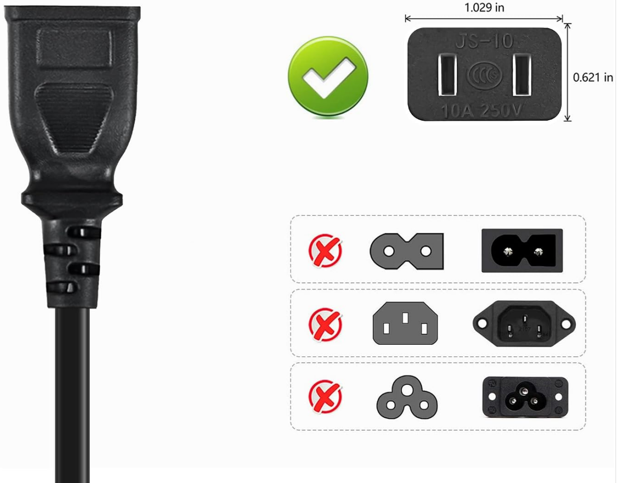
Figure 3: Diagram illustrating the compatible two-slot female receptacle (JS-10, 10A 250V) and examples of incompatible plug types.
