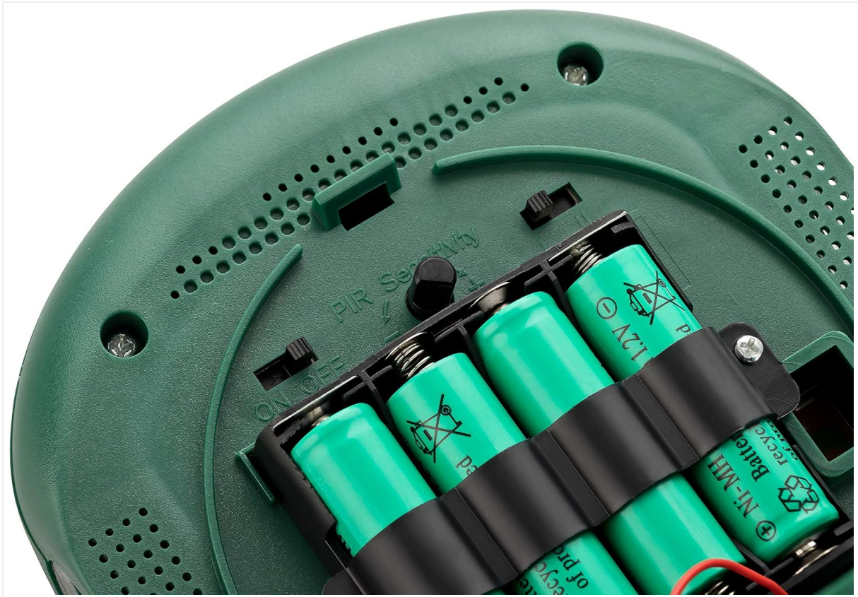
Image: View of the battery compartment with Ni-MH batteries installed.
