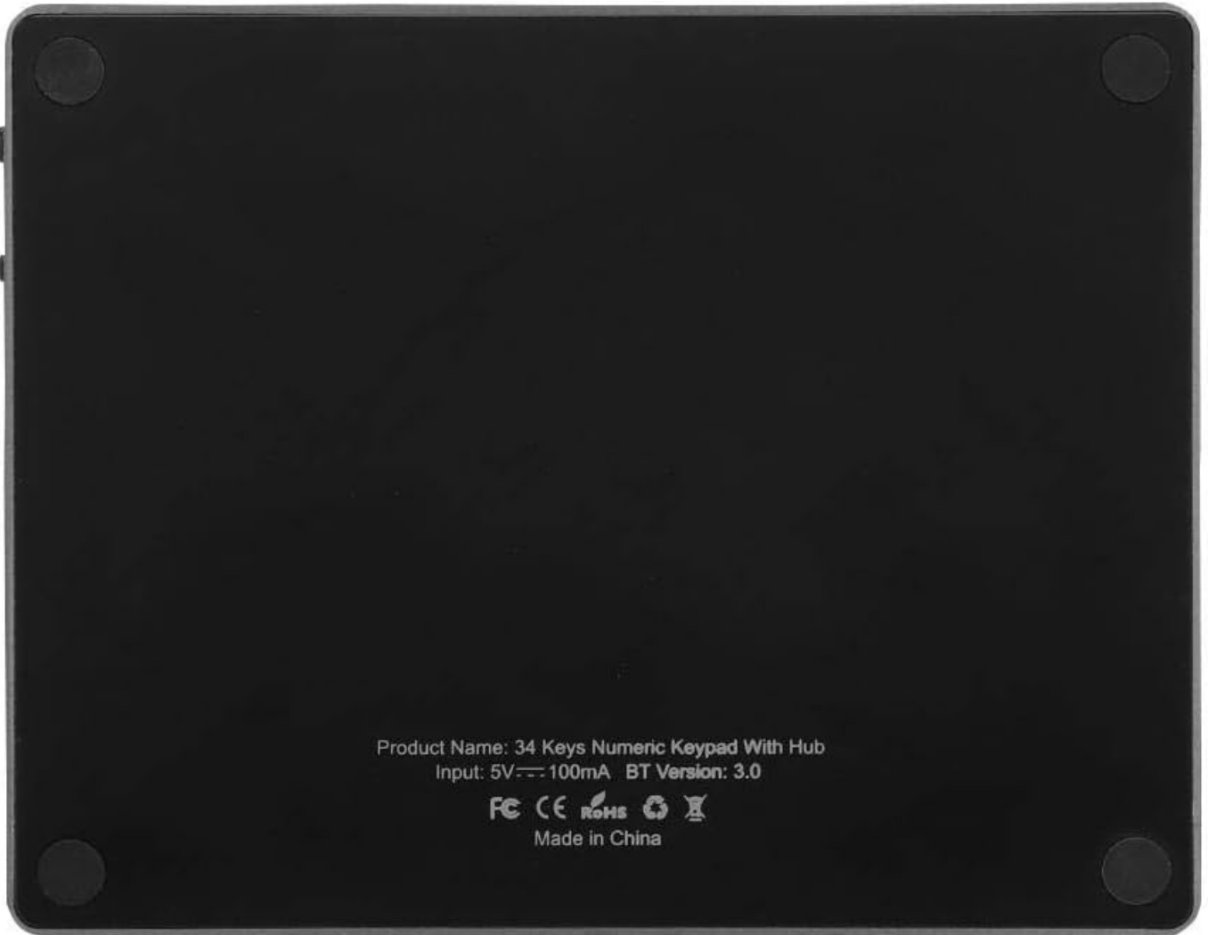
Figure 6: Keypad Bottom View with Specifications
