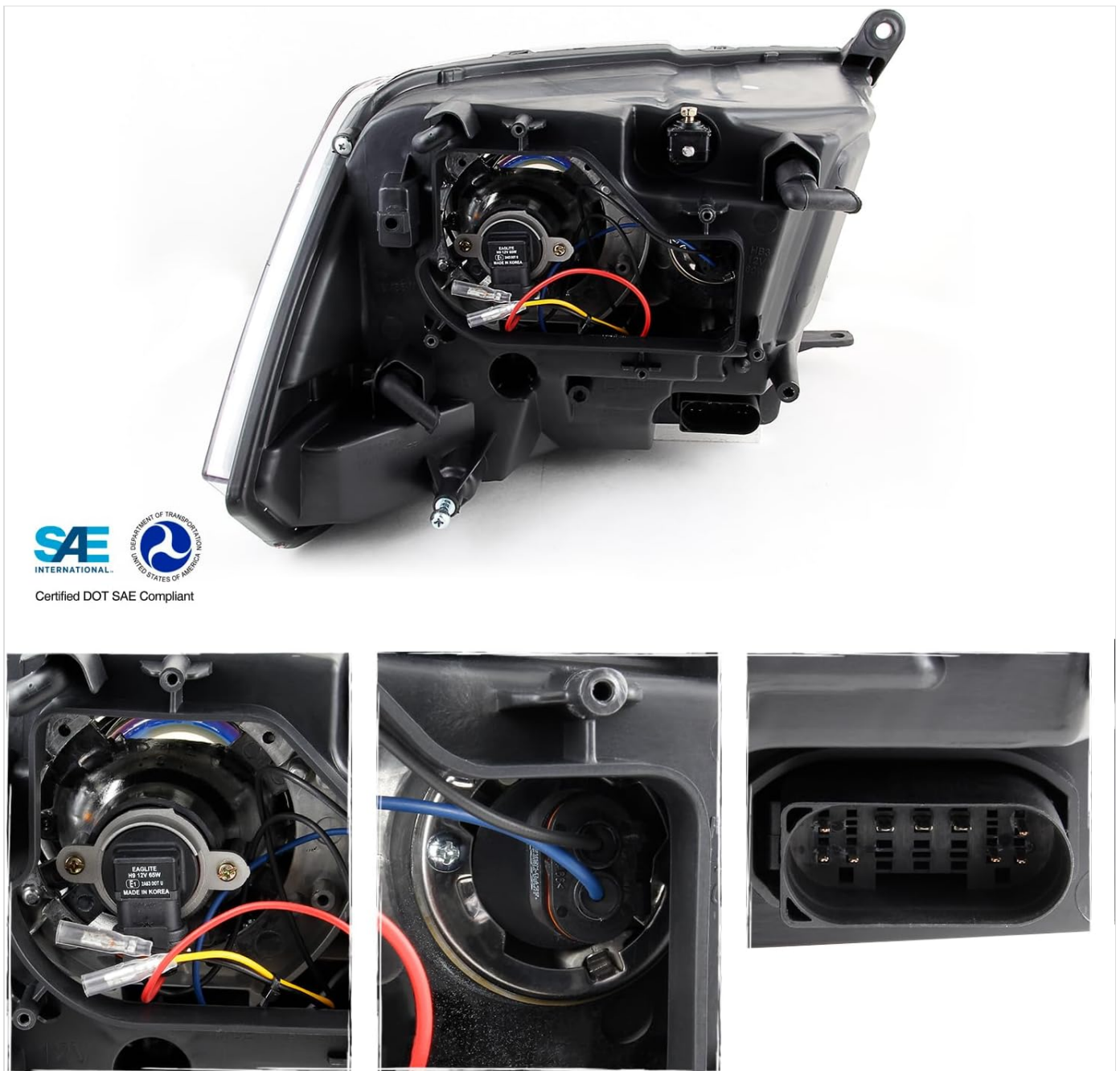
Image: Rear view of the AKKON headlight assembly, detailing the wiring harness and bulb access points.
