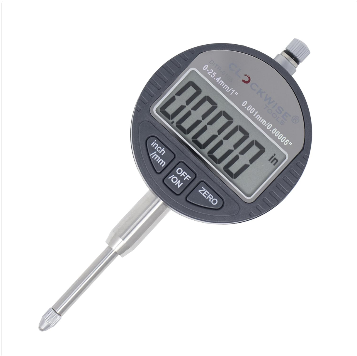
Figure 3.1: Front view of the Clockwise Tools DITR-0105N Digital Indicator, showing the LCD display and control buttons. This image illustrates the main body of the digital indicator, including the large digital readout, the 'inch/mm' button for unit conversion, the 'OFF/ON' button for power, and the 'ZERO' button for setting a reference point. The measuring spindle extends from the bottom.
