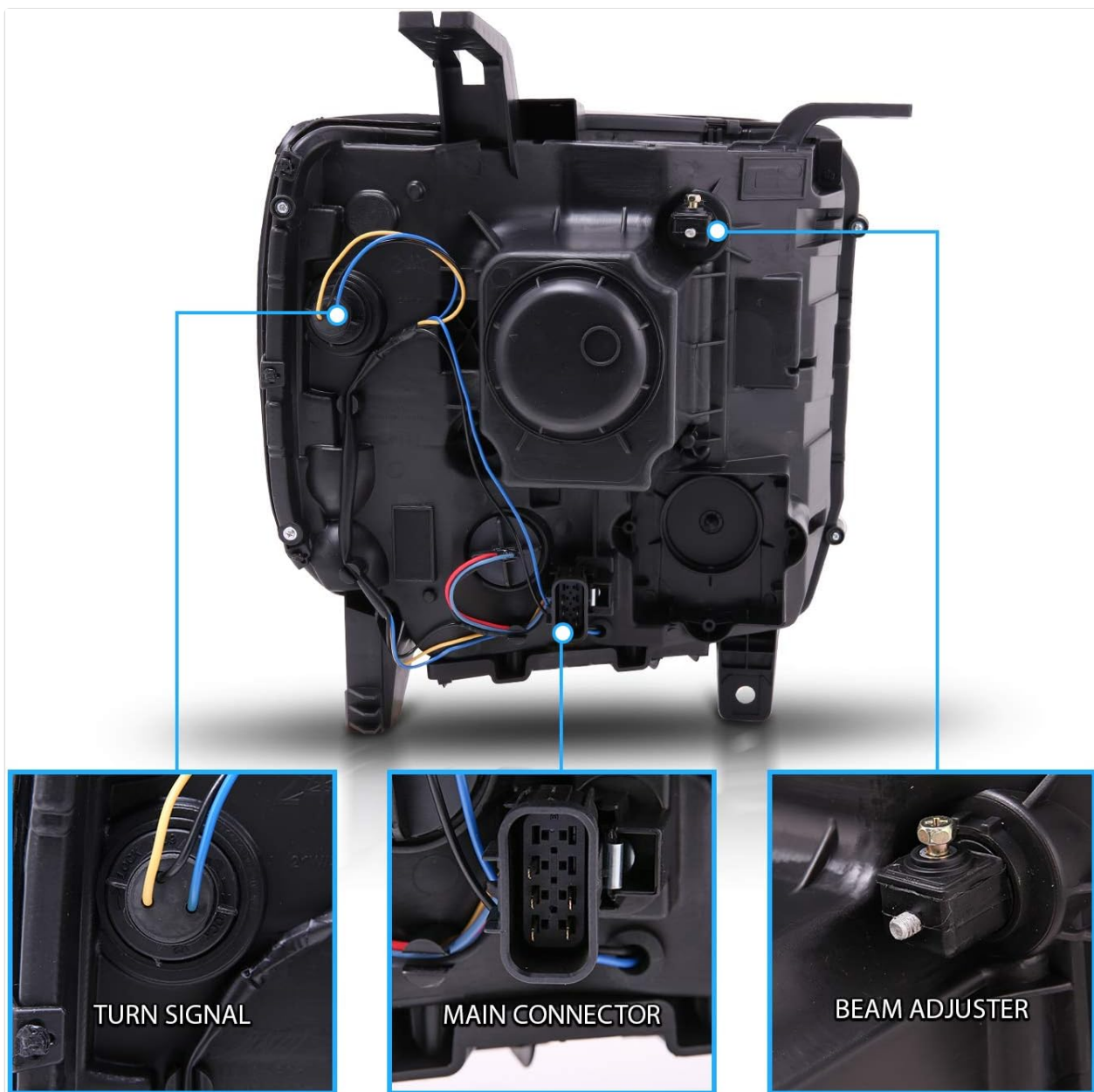
Image 4.1: Rear view of the headlight assembly highlighting electrical connections and adjustment points.
