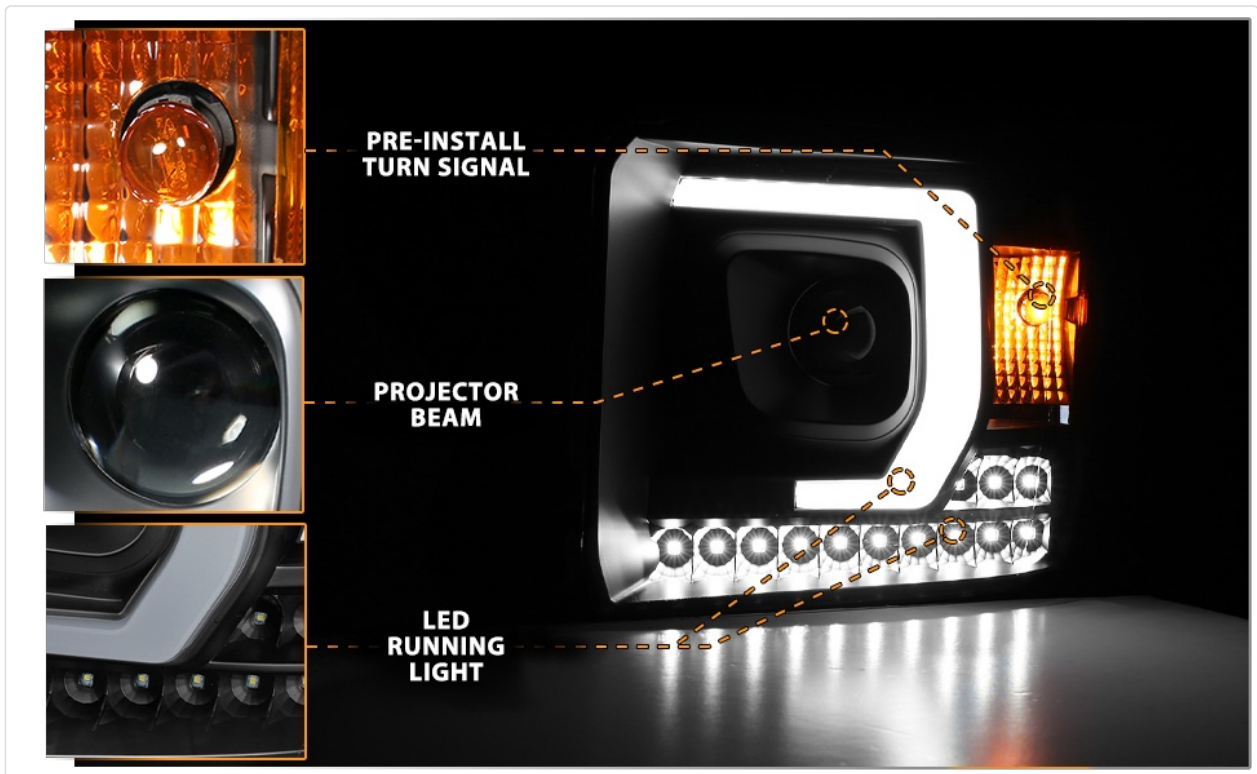
Image 5.2: The C-shape LED light bar serving as a Daytime Running Light.
