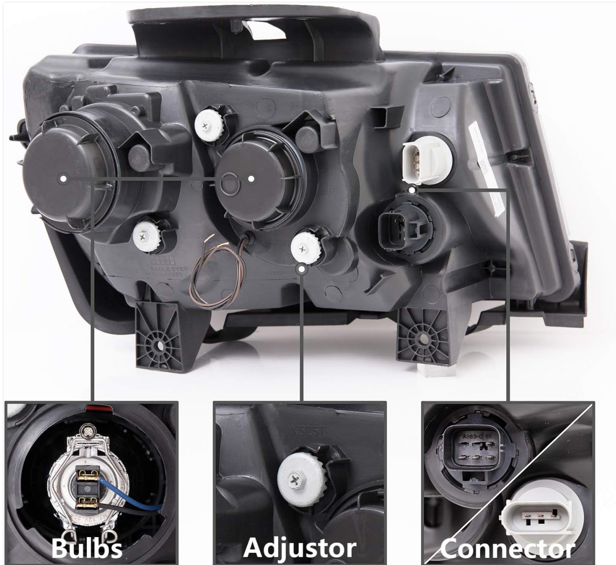
Image 3: Rear view of the headlight assembly, highlighting bulb access points, adjusters, and electrical connectors.
