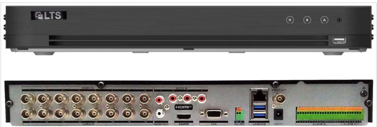
Figure 4.2: Rear panel connections. This image details the rear panel of the DVR, highlighting the BNC video input ports (1-16), audio input/output, HDMI, VGA, LAN, USB, and power input ports.
