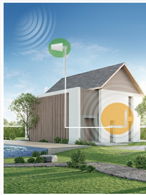
Image 3.2: Visual representation of the kit contents: (1) Outdoor Antenna, (2) Booster, (3) Indoor Antenna, (4) Coaxial Cable, (5) Power Supply.
