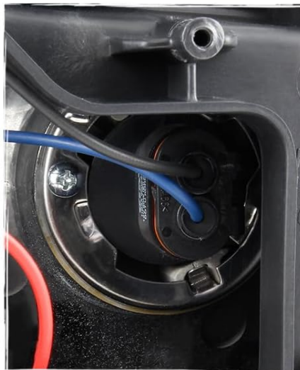
Image 5.2: Rear view of Headlight Assembly with wiring.
