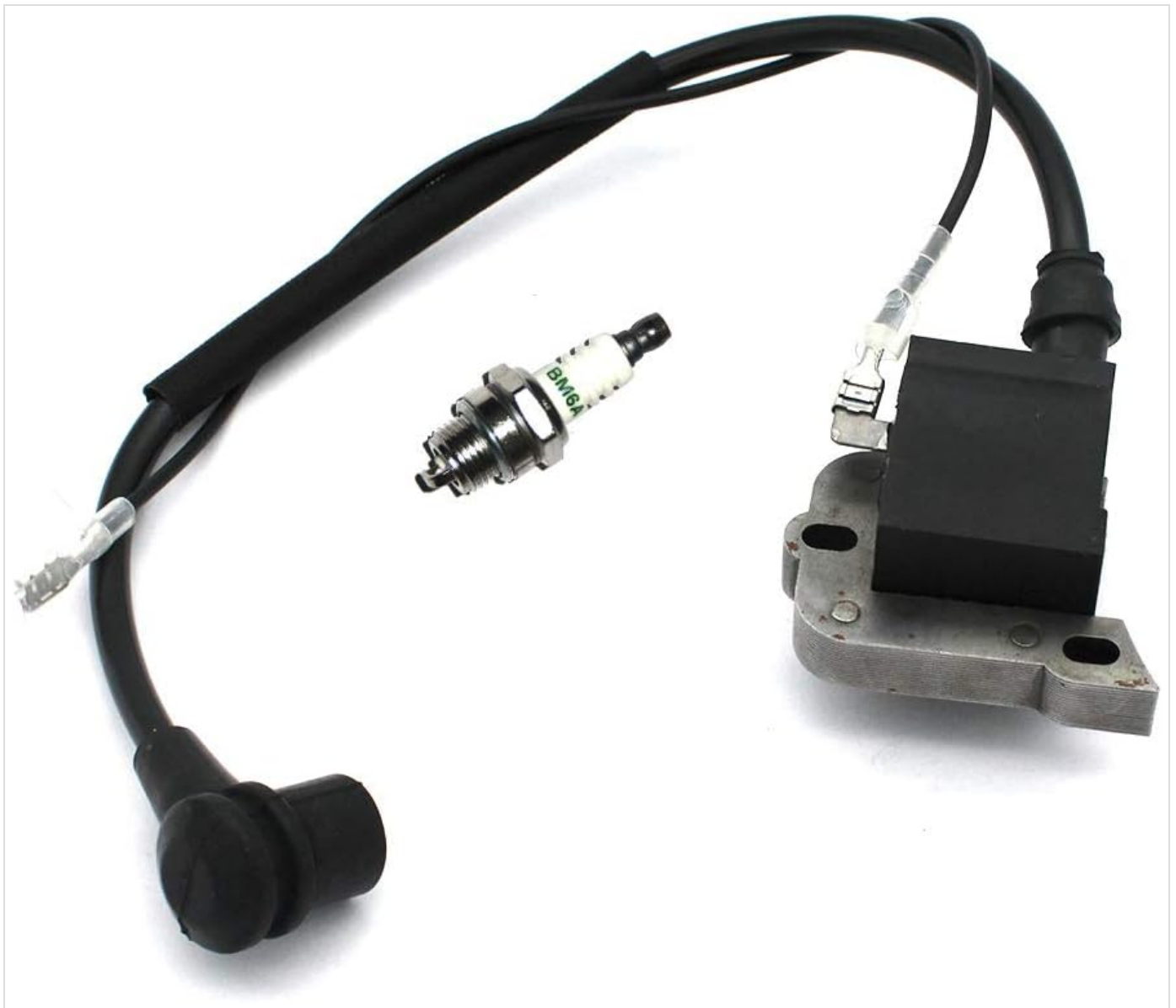
Image: Another view of the ignition coil and spark plug, showing the connecting wires and terminals.
