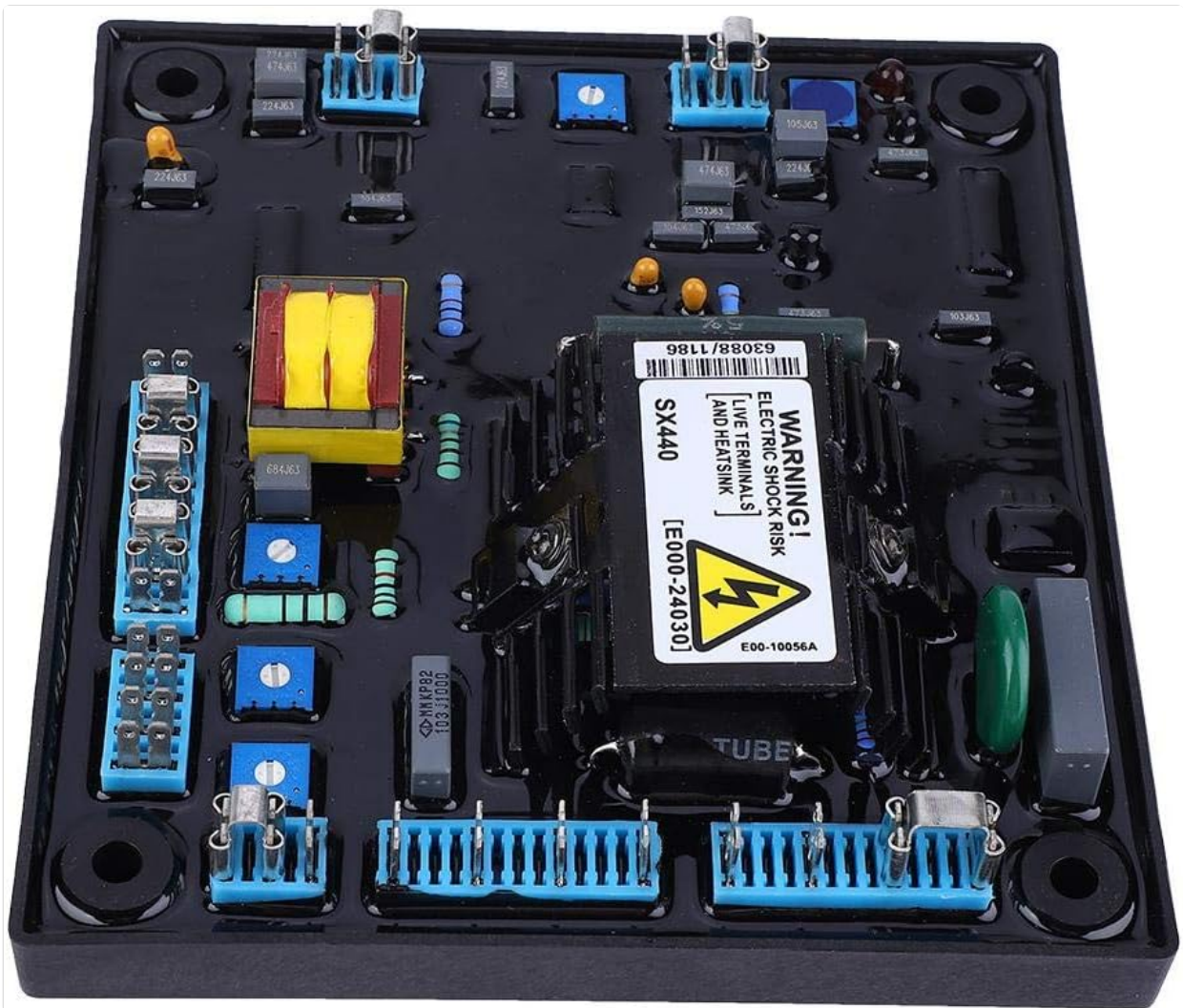
Image 5.1: Close-up view of the SX440 AVR, detailing the terminal blocks for wiring connections and adjustment potentiometers.
