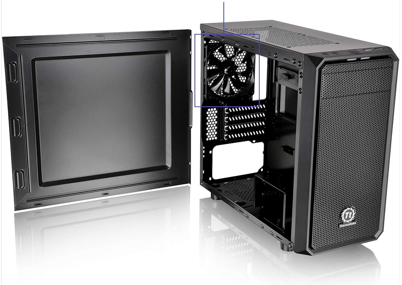
Figure 3: View of the chassis with the side panel removed, highlighting the pre-installed 120mm rear exhaust fan.
