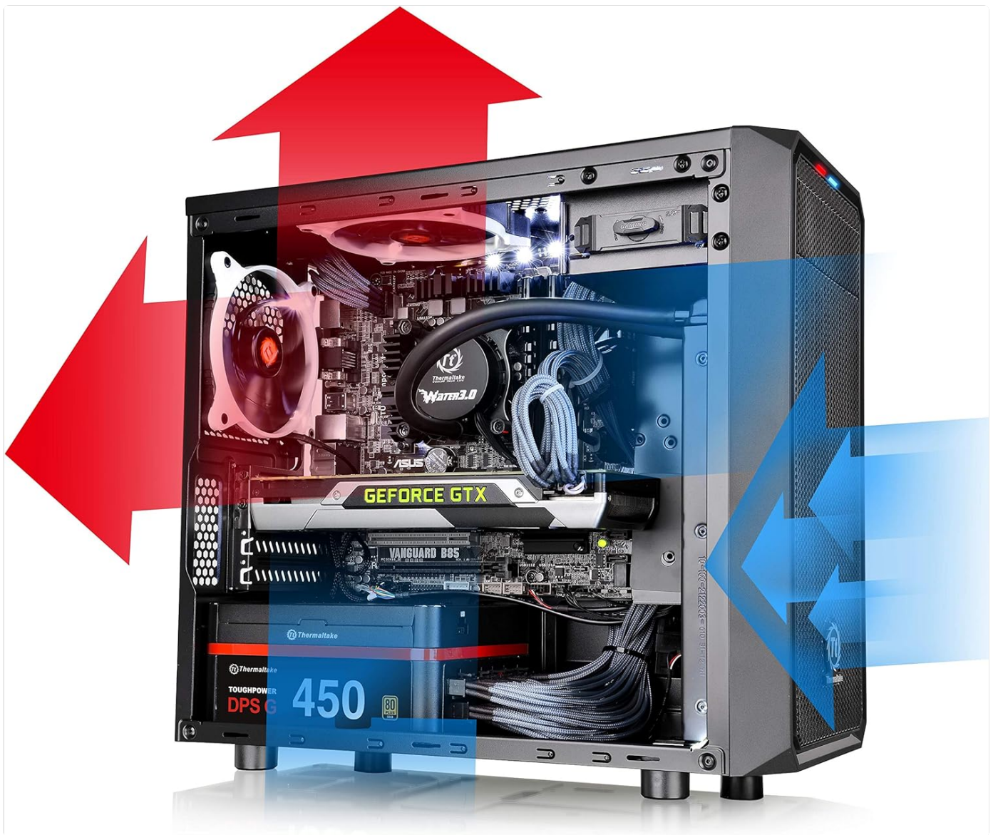
Figure 6: Diagram illustrating the airflow path within the Thermaltake Versa H15 chassis, showing intake and exhaust areas.
