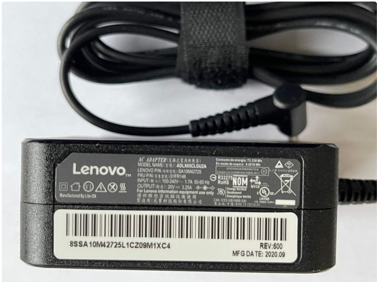
Figure 3: Detailed view of the adapter's label, showing electrical specifications and certifications.
