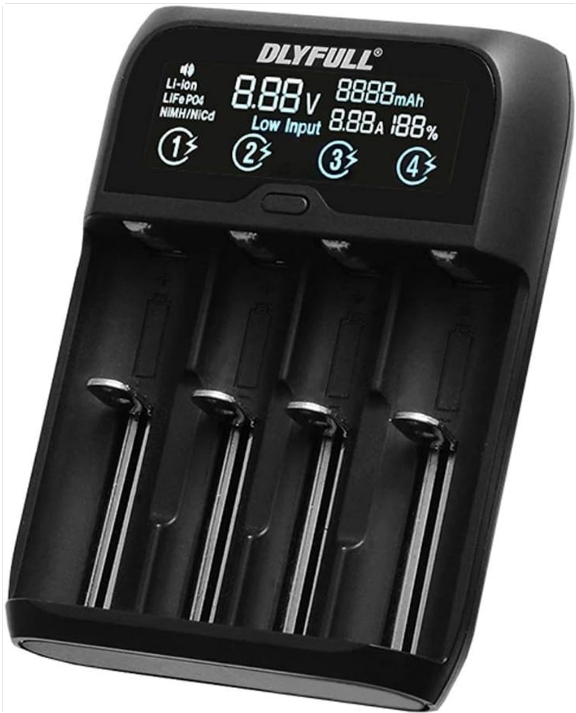
Figure 3.1: Front view of the DLYFULL UM4 Multi-Charger, showing the digital display and four independent battery charging slots.
