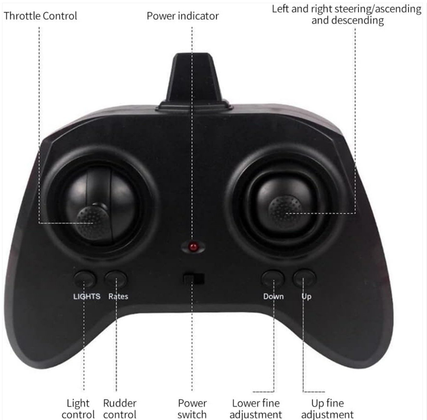
Image 4.1: Remote Control Layout and Functions.
