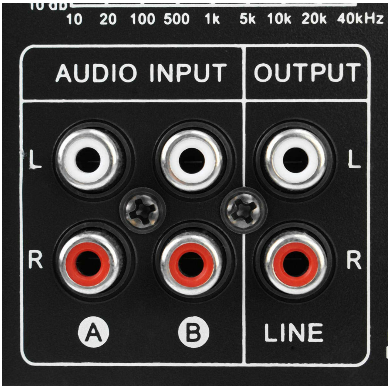
Figure 4: Detailed view of the "AUDIO INPUT" (A, B) and "OUTPUT" (LINE) RCA jacks.
