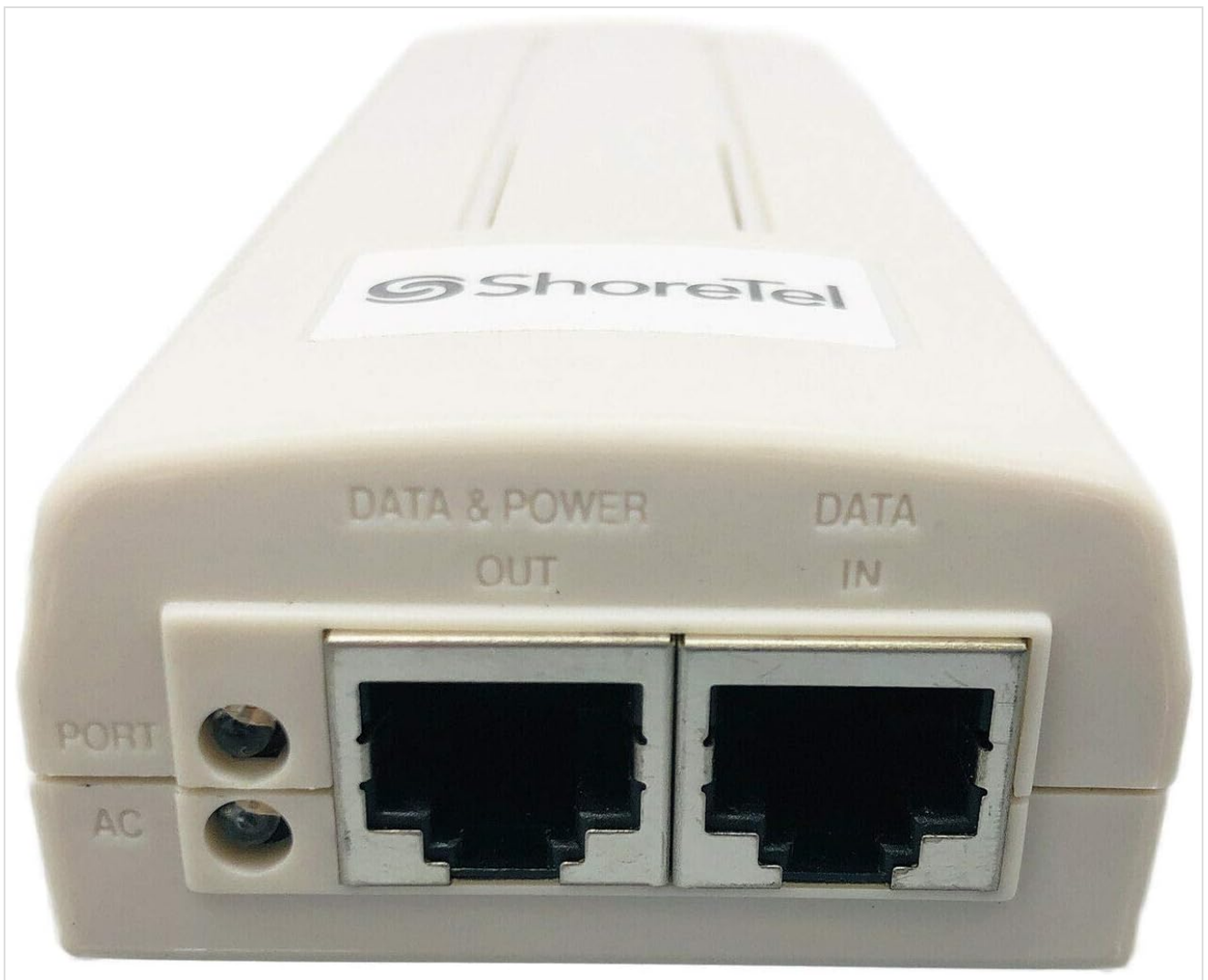
Figure 2: Rear view of the PowerDsine 3001 PoE Injector showing the "DATA IN" port (for connection to a network switch/router), the "DATA & POWER OUT" port (for connection to a PoE-compatible device), and the AC power input.
