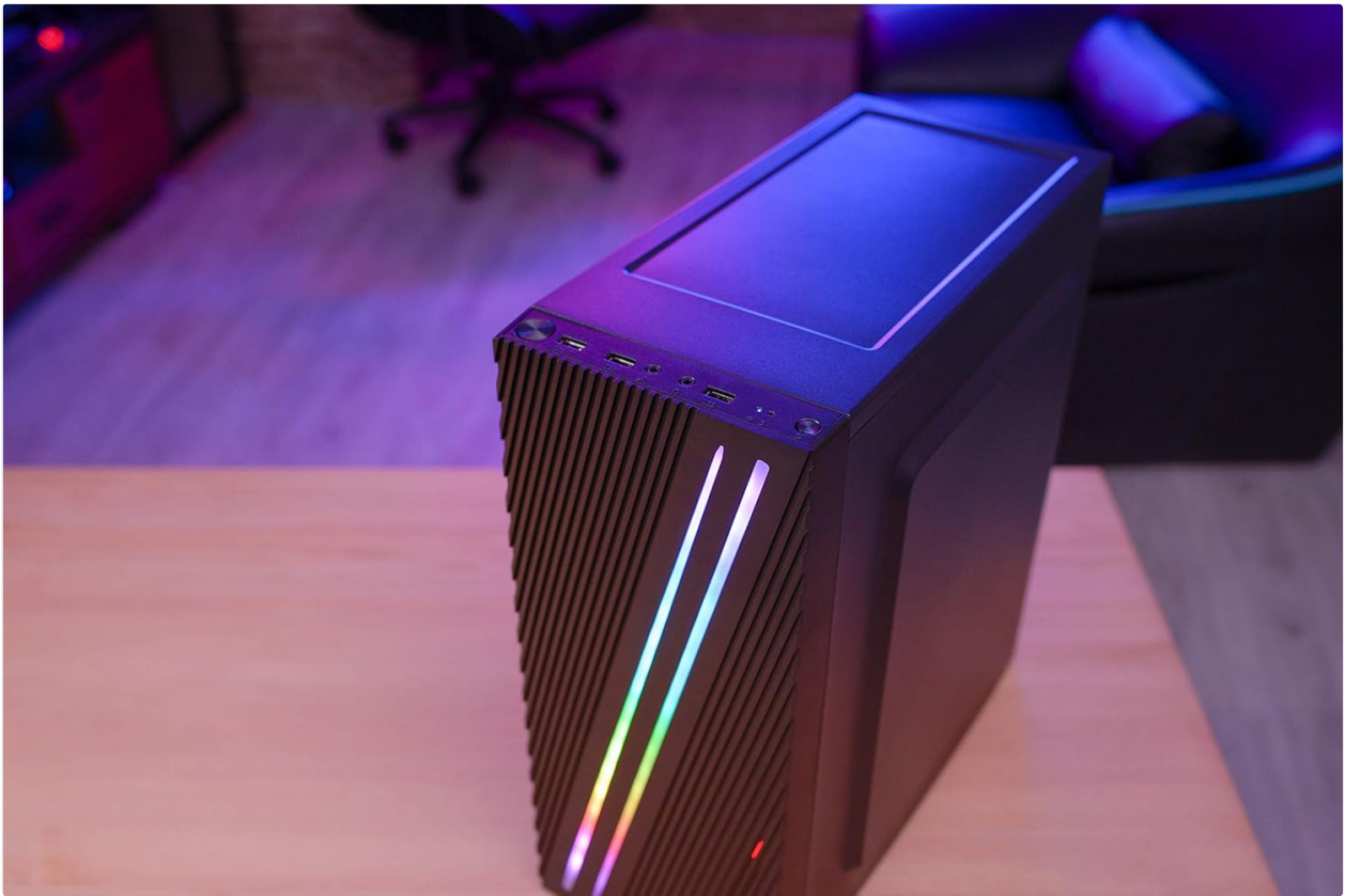
Figure 4.3: Close-up of the front I/O panel, showing the power button, LED control button, USB 3.0 port, two USB 2.0 ports, and HD audio/microphone jacks.
