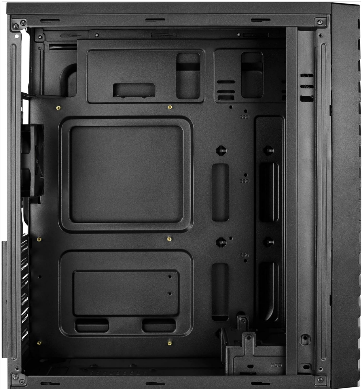
Figure 4.4: Internal view of the Aerocool Streak PC case, showing the motherboard tray, drive bays, and cable routing cutouts.
