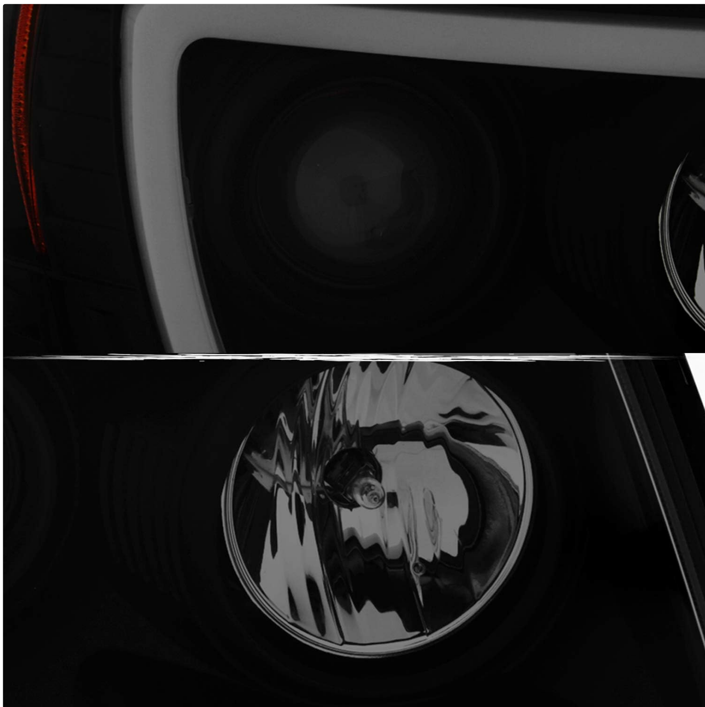
Image: Detailed view of the projector lens and the distinctive U-Tube LED bar within the headlight assembly.
